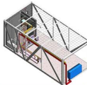
PHASE 3 – MEP INSTALLATION IN FACTORY
