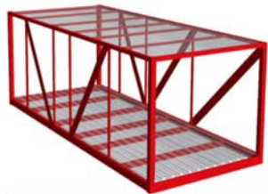
PHASE 1 - MANUFACTURED MODULAR STEEL FRAME
