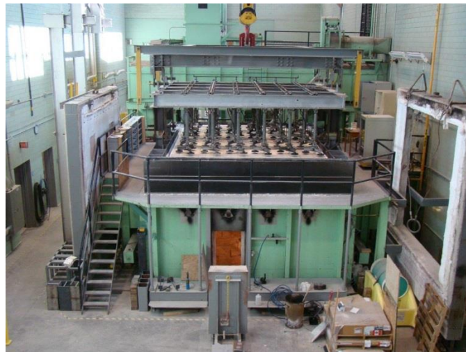
Figure 1: NRC full-scale floor furnace facility
