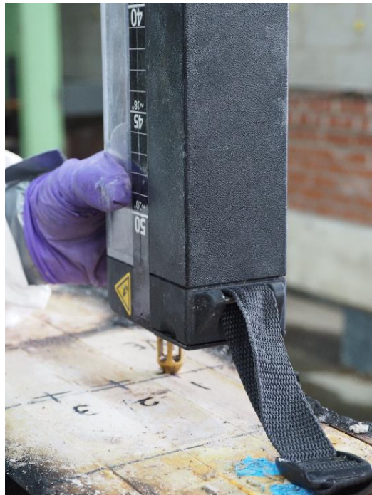
(c) Measurement of char depth of the Beam after the test
