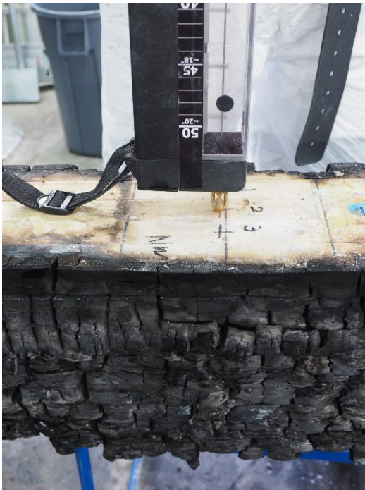
(c) Measurement of char depth of the Beam after the test
