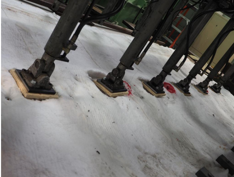
Figure 5: Top of the furnace after the placing the Beam
