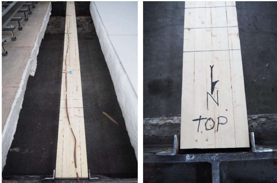
Figure 3: L-section rotation preventive mechanism
