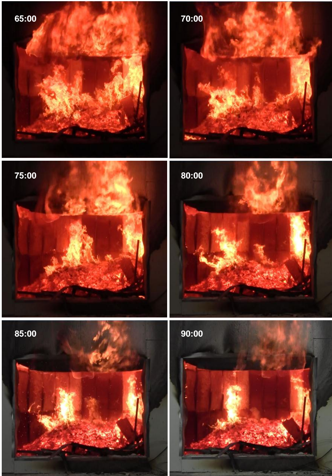
Figure 21. Video graphic captures of fire development (65-90 min).
