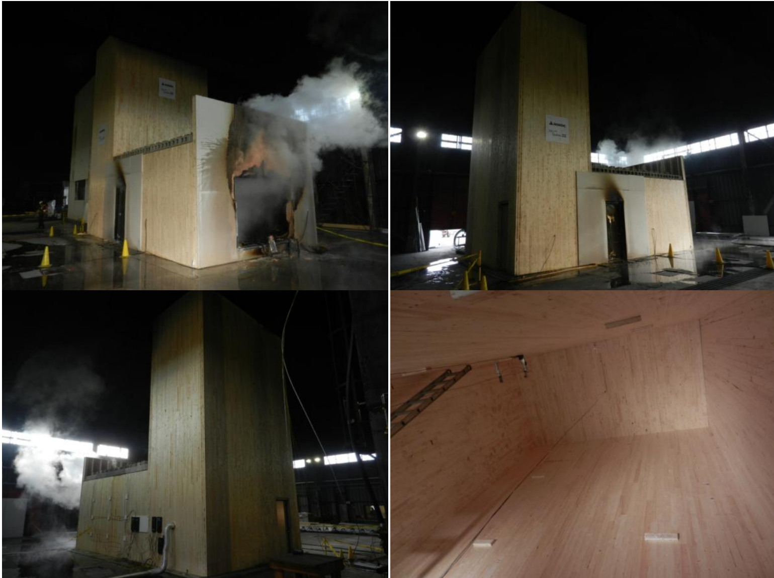
Figure 33. Outside of the demonstration structure and inside of the stair/elevator shaft after the fire demonstration.
