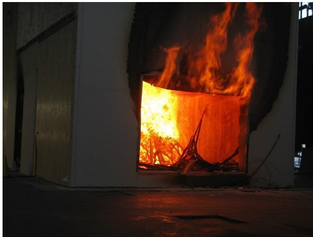
c) After 45 min, steel channels have fallen
