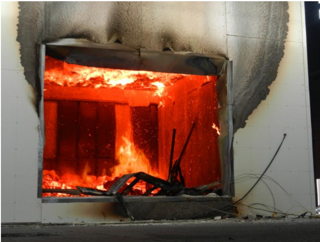
Figure 28. Double layer of gypsum board and rigid mineral wool fibre insulation remained on the apartment wall until end of demonstration.
