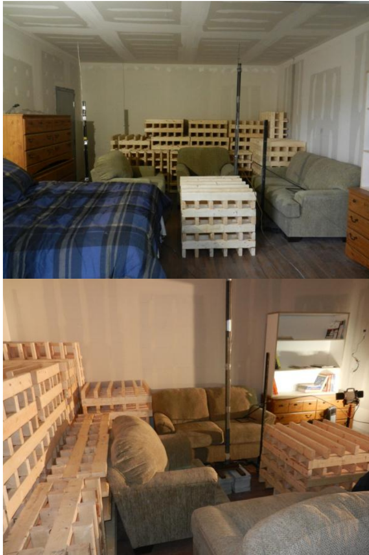
Figure 12. Photographs of fuel arrangement in the fire compartment.
