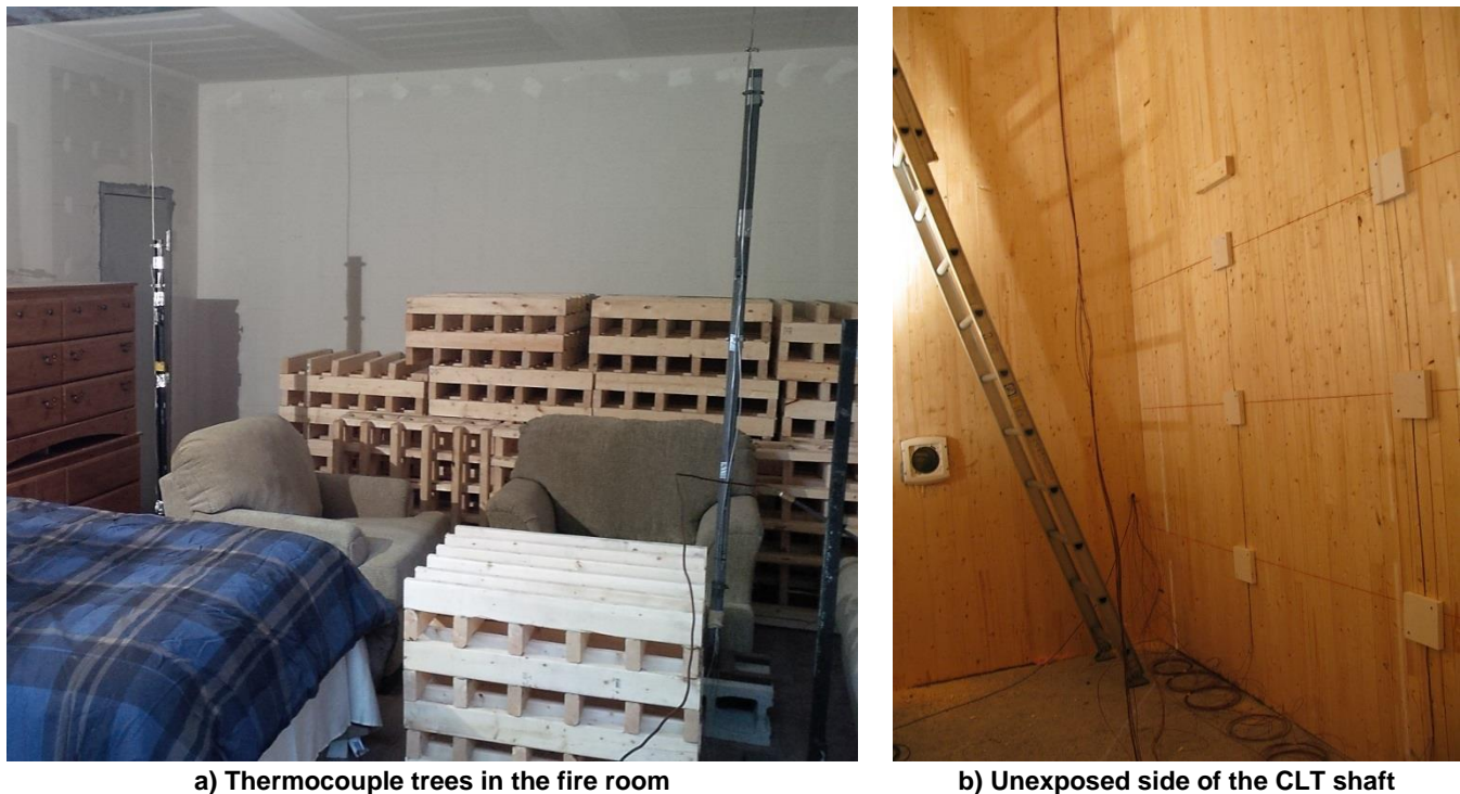
Figure 8. Instrumentation of the structure
