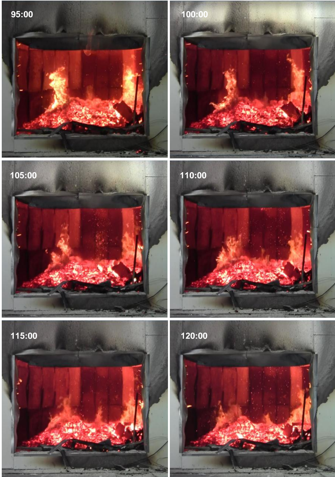
Figure 22. Video graphic captures of fire development (95-120 min).
